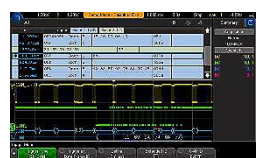
Figure 19. Multi-bus time aligned decode.
