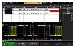
Figure 17. CAN-FD decode and trigger.
