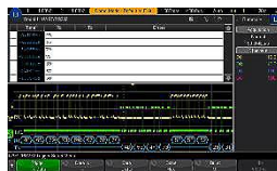
Figure 16. RS232 decode and trigger.
